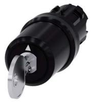
key-operated switch Siemens, 22 mm, round, plastic, lock number SSG10, with 2 keys, 3 switch positions I>O<II, momentary contact on the left, latching on the right, actuating angle 2x45°, 10:30h/12h/13:30h, key removal O+II, with laser labeling, lower case
