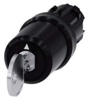
key-operated switch Siemens, 22 mm, round, plastic, lock number SSG10, with 2 keys, 3 switch positions I>O<II, momentary contact on the left, latching on the right, actuating angle 2x45°, 10:30h/12h/13:30h, key removal II, with laser labeling, upper case and lower case, always upper case at the beginning of the word
