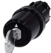
key-operated switch Siemens, 22 mm, round, plastic, lock number SSG10, with 2 keys, 3 switch positions I>O<II, momentary contact on the left, latching on the right, actuating angle 2x45°, 10:30h/12h/13:30h, key removal II, with laser labeling, upper case
