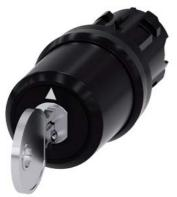
key-operated switch Siemens, 22 mm, round, plastic, lock number SSG10, with 2 keys, 3 switch positions I-O<II, left latching, momentary contact type on the right, actuating angle 2x45°, 10:30h/12h/13:30h, key removal O+I Z=50-unit packaging
