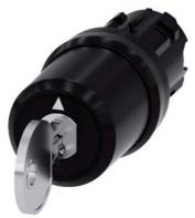
key-operated switch Siemens, 22 mm, round, plastic, lock number SSG10, with 2 keys, 3 switch positions I-O<II, left latching, momentary contact type on the right, actuating angle  $2x45^{\circ}$ , 10:30h/12h/13:30h, key removal I, with laser labeling, upper case
