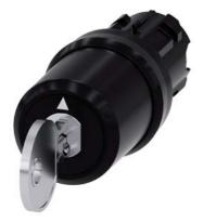
key-operated switch Siemens, 22 mm, round, plastic, lock number SSG10, with 2 keys, 3 switch positions I>O<II, momentary contact type, actuating angle 2x45°, 10:30h/12h/13:30h, key removal O, with laser labeling, inscription or symbol customer-specific selection with SIRIUS ACT configurator (CIN)
