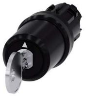
key-operated switch Siemens, 22 mm, round, plastic, lock number SSG10, with 2 keys, 3 switch positions I>O<II, momentary contact type, actuating angle 2x45°, 10:30h/12h/13:30h, key removal O, with laser labeling, lower case
