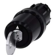
key-operated switch Siemens, 22 mm, round, plastic, lock number SSG10, with 2 keys, 3 switch positions I-O-II, latching, actuating angle  $2x45^{\circ}$ , 10:30h/12h/13:30h, key removal O+I Z=50-unit packaging
