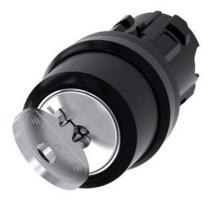
RONIS key-operated switch, 22 mm, round, plastic, lock number 455, with 2 keys, 2 switch positions O-I, latching, actuating angle 90°, 10:30h/13:30h, key removal O, with laser labeling, upper case and lower case, always upper case at the beginning of the word
