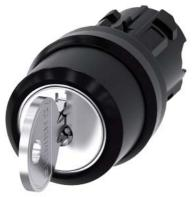
RONIS key-operated switch, 22 mm, round, plastic, lock number SB30, with 2 keys, 3 switch positions >O<II, momentary contact on the left, latching on the right, actuating angle 2x45°, 10:30h/12h/13:30h, Key removal O+II, possible special locks: SB31, 421, 455 Z=50-unit packaging
