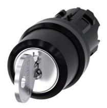
RONIS key-operated switch, 22 mm, round, plastic, lock number SB30, with 2 keys, 3 switch positions I>O<II, momentary contact on the left, latching on the right, actuating angle 2x45°, 10:30h/12h/13:30h, Key removal II, possible special locks: SB31, 421, 455, with laser labeling, lower case
