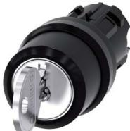
RONIS key-operated switch, 22 mm, round, plastic, lock number SB30, with 2 keys, 3 switch positions I-O<II, left latching, right momentary contact type, actuating angle 2x45°, 10:30h/12h/13:30h, key removal I, possible special locks: SB31, 421, 455, with laser labeling, lower case
