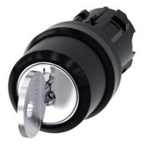
RONIS key-operated switch, 22 mm, round, plastic, special lock, with 2 keys, 3 switch positions I-O<II, left latching, right momentary contact type, actuating angle 2x45°, 10:30h/12h/13:30h, key removal I, possible special locks: SB31, 421, 455
