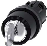
RONIS key-operated switch, 22 mm, round, plastic, lock number SB30, with 2 keys, 3 switch positions I>O<II, momentary contact type, actuating angle 2x45°, 10:30h/12h/13:30h, key removal O, possible special locks: SB31, 421, 455, with laser labeling, upper case
