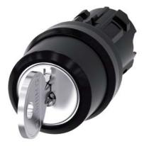
RONIS key-operated switch, 22 mm, round, plastic, lock number SB30, with 2 keys, 3 switch positions I-O-II, latching, actuating angle 2x45°, 10:30h/12h/13:30h, key removal I, possible special locks: SB31, 421, 455, with laser labeling, upper case and lower case, always upper case at beginning of line
