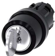
RONIS key-operated switch, 22 mm, round, plastic, lock number SB30, with 2 keys, 3 switch positions I-O-II, latching, actuating angle 2x45°, 10:30h/12h/13:30h, key removal I, possible special locks: SB31, 421, 455 Z=50-unit packaging
