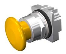
30mm Command/52, Chrome Finish Heavy Duty, Watertight/Oiltight Metal Operator, Round Push-Pull Operator Non-Illuminated Mushroom Head Cap Small 1 3/4" (44.5 mm) Plastic, Yellow 2 Position Maintained, Pull-to-Release UL Listed, CSA Certified NEMA 1,3,3R,4,4X,12,13 & Automotive Standards
