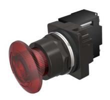
30mm BlackMax, Epoxy Coated Corrosion Resistant Metal Operator, Round Illuminated Twist-to-Release Transformer type, 480V AC Incandescent Lamp Mushroom Head Cap Small 1.79" (45 mm) Plastic Cap, Red 2 Position Maintained, Twist-to-Release UL Listed, CSA Certified NEMA 1,3,3R,4,4X,12,13 & Automotive Standards
