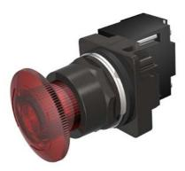
30mm BlackMax, Epoxy Coated Corrosion Resistant Metal Operator, Round Illuminated Twist-to-Release Transformer type, 240V AC LED Lamp Mushroom Head Cap Small 1.79" (45 mm) Plastic Cap, Red 2 Position Maintained, Twist-to-Release UL Listed, CSA Certified NEMA 1,3,3R,4,4X,12,13 & Automotive Standards
