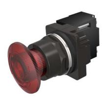
30mm BlackMax, Epoxy Coated Corrosion Resistant Metal Operator, Round Illuminated Twist-to-Release Transformer type, 120V AC LED Lamp Mushroom Head Cap Small 1.79" (45 mm) Plastic Cap, Red 2 Position Maintained, Twist-to-Release UL Listed, CSA Certified NEMA 1,3,3R,4,4X,12,13 & Automotive Standards
