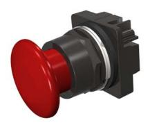
30mm BlackMax, Epoxy Coated Corrosion Resistant Metal Operator, Round Push-Pull Operator Non-Illuminated Mushroom Head Cap Small 1 3/4" (44.5 mm) Plastic, Red 3 Position Pull-Momentary/Push-Maintained UL Listed, CSA Certified NEMA 1,3,3R,4,4X,12,13 & Automotive Standards
