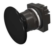
30mm BlackMax, Epoxy Coated Corrosion Resistant Metal Operator, Round Push-Pull Operator Non-Illuminated Mushroom Head Cap Large 2 1/2" (63.5 mm) Plastic, Black 3 Position Pull-Momentary/Push-Maintained UL Listed, CSA Certified NEMA 1,3,3R,4,4X,12,13 & Automotive Standards
