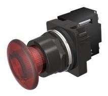
30mm BlackMax, Epoxy Coated Corrosion Resistant Complete Metal Unit Illuminated Push-Pull Operator Transformer type, 600V AC Incandescent Lamp Mushroom Head Cap Small 1 3/4" (44.5 mm) Plastic, Red 3 Position Pull-Momentary/Push-Maintained UL Listed, CSA Certified NEMA 1,3,3R,4,4X,12,13 & Automotive Standards
