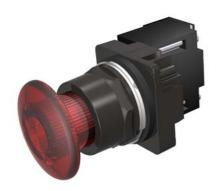
30mm BlackMax, Epoxy Coated Corrosion Resistant Complete Metal Unit Illuminated Push-Pull Operator Transformer type, 480V AC Incandescent Lamp Mushroom Head Cap Small 1 3/4" (44.5 mm) Plastic, Red 3 Position Pull-Momentary/Push-Maintained UL Listed, CSA Certified NEMA 1,3,3R,4,4X,12,13 & Automotive Standards
