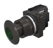
30mm BlackMax, Epoxy Coated Corrosion Resistant Complete Metal Unit Illuminated Push-Pull Operator Transformer type, 480V AC Incandescent Lamp Mushroom Head Cap Small 1 3/4" (44.5 mm) Metal, Black with Green Lens 3 Position Pull-Momentary/Push-Maintained UL Listed, CSA Certified NEMA 1,3,3R,4,4X,12,13 & Automotive Standards
