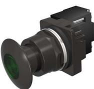
30mm BlackMax, Epoxy Coated Corrosion Resistant Complete Metal Unit Illuminated Push-Pull Operator Transformer type, 240V AC Incandescent Lamp Mushroom Head Cap Small 1 3/4" (44.5 mm) Metal, Black with Green Lens 3 Position Pull-Momentary/Push-Maintained UL Listed, CSA Certified NEMA 1,3,3R,4,4X,12,13 & Automotive Standards
