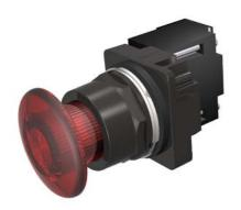
30mm BlackMax, Epoxy Coated Corrosion Resistant Complete Metal Unit Illuminated Push-Pull Operator Full Voltage, 12V AC/DC Incandescent Lamp Mushroom Head Cap Small 1 3/4" (44.5 mm) Plastic, Red 3 Position Pull-Momentary/Push-Maintained UL Listed, CSA Certified NEMA 1,3,3R,4,4X,12,13 & Automotive Standards
