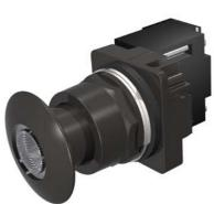
30mm BlackMax, Epoxy Coated Corrosion Resistant Complete Metal Unit Illuminated Push-Pull Operator Transformer type, 480V AC Incandescent Lamp Mushroom Head Cap Small 1 3/4" (44.5 mm) Metal, Black with Clear Lens 3 Position Momentary UL Listed, CSA Certified NEMA 1,3,3R,4,4X,12,13 & Automotive Standards
