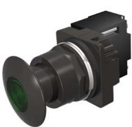
30mm BlackMax, Epoxy Coated Corrosion Resistant Complete Metal Unit Illuminated Push-Pull Operator Transformer type, 240V AC Incandescent Lamp Mushroom Head Cap Small 1 3/4" (44.5 mm) Metal, Black with Green Lens 3 Position Momentary UL Listed, CSA Certified NEMA 1,3,3R,4,4X,12,13 & Automotive Standards
