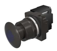
30mm BlackMax, Epoxy Coated Corrosion Resistant Complete Metal Unit Illuminated Push-Pull Operator Transformer type, 120V AC Incandescent Lamp Mushroom Head Cap Small 1 3/4" (44.5 mm) Metal, Black with Blue Lens 3 Position Momentary UL Listed, CSA Certified NEMA 1,3,3R,4,4X,12,13 & Automotive Standards
