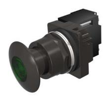
30mm BlackMax, Epoxy Coated Corrosion Resistant Complete Metal Unit Illuminated Push-Pull Operator Full Voltage, 24V AC/DC Incandescent Lamp Mushroom Head Cap Small 1 3/4" (44.5 mm) Metal, Black with Green Lens 3 Position Momentary UL Listed, CSA Certified NEMA 1,3,3R,4,4X,12,13 & Automotive Standards
