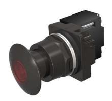
30mm BlackMax, Epoxy Coated Corrosion Resistant Complete Metal Unit Illuminated Push-Pull Operator Full Voltage, 24V AC/DC Incandescent Lamp Mushroom Head Cap Small 1 3/4" (44.5 mm) Metal, Black with Red Lens 3 Position Momentary UL Listed, CSA Certified NEMA 1,3,3R,4,4X,12,13 & Automotive Standards
