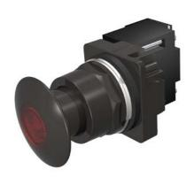
30mm BlackMax, Epoxy Coated Corrosion Resistant Complete Metal Unit Illuminated Push-Pull Operator Transformer type, 480V AC Incandescent Lamp Mushroom Head Cap Small 1 3/4" (44.5 mm) Metal, Black with Red Lens 2 Position Maintained, Pull-to-Release UL Listed, CSA Certified NEMA 1,3,3R,4,4X,12,13 & Automotive Standards
