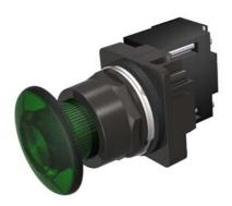
30mm BlackMax, Epoxy Coated Corrosion Resistant Complete Metal Unit Illuminated Push-Pull Operator Transformer type, 240V AC LED Lamp Mushroom Head Cap Small 1 3/4" (44.5 mm) Plastic, Green 2 Position Maintained, Pull-to-Release UL Listed, CSA Certified NEMA 1,3,3R,4,4X,12,13 & Automotive Standards
