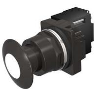
30mm BlackMax, Epoxy Coated Corrosion Resistant Complete Metal Unit Illuminated Push-Pull Operator Transformer type, 240V AC LED Lamp Mushroom Head Cap Small 1 3/4" (44.5 mm) Metal, Black with White Lens 2 Position Maintained, Pull-to-Release UL Listed, CSA Certified NEMA 1,3,3R,4,4X,12,13 & Automotive Standards
