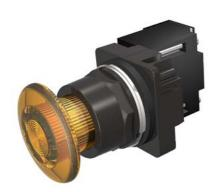
30mm BlackMax, Epoxy Coated Corrosion Resistant Complete Metal Unit Illuminated Push-Pull Operator Full Voltage, 120V AC/DC Incandescent Lamp Mushroom Head Cap Small 1 3/4" (44.5 mm) Plastic, Amber 2 Position Maintained, Pull-to-Release UL Listed, CSA Certified NEMA 1,3,3R,4,4X,12,13 & Automotive Standards
