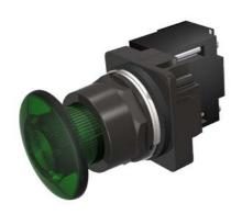
30mm BlackMax, Epoxy Coated Corrosion Resistant Complete Metal Unit Illuminated Push-Pull Operator Full Voltage, 24V AC/DC LED Lamp Mushroom Head Cap Small 1 3/4" (44.5 mm) Plastic, Green 2 Position Maintained, Pull-to-Release UL Listed, CSA Certified NEMA 1,3,3R,4,4X,12,13 & Automotive Standards
