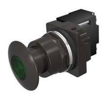
30mm BlackMax, Epoxy Coated Corrosion Resistant Complete Metal Unit Illuminated Push-Pull Operator Full Voltage, 24V AC/DC Incandescent Lamp Mushroom Head Cap Small 1 3/4" (44.5 mm) Metal, Black with Green Lens 2 Position Maintained, Pull-to-Release UL Listed, CSA Certified NEMA 1,3,3R,4,4X,12,13 & Automotive Standards
