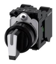
Selector switch, illuminable, 22 mm, round, plastic, white, selector switch, short, 3 switch positions I>O<II, momentary contact type, 10:30h/12h/13:30h, with holder, 1 NO, 1 NO, Spring-type terminal
