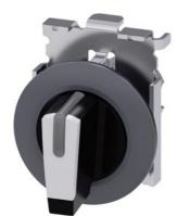
Selector switch, illuminable, 30 mm, round, metal, matte, white, selector switch, short, front ring for flush installation, 3 switch positions I>O<II, momentary contact type, actuating angle  $2x45^{\circ}$ , 10:30h/12h/13:30h
