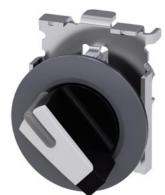
Selector switch, illuminable, 30 mm, round, metal, matte, white, selector switch, short, front ring for flush installation, 2 switch positions O<I, momentary contact type, Actuating angle 45°, 10:30h/12h
