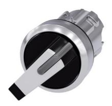
Illuminable selector switch, 22 mm, round, metal shiny, white, Selector switch short, 2 switch positions O<I, momentary contact type, Actuating angle 45°, 13:30h/15h
