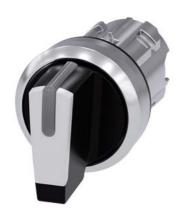
Selector switch, illuminable, 22 mm, round, metal, shiny, white, selector switch, short, 3 switch positions I>O<II, momentary contact type, actuating angle 2x45°, 10:30h/12h/13:30h
