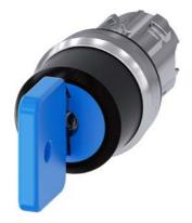
Key-operated switch O.M.R, 22 mm, round, metal, shiny, lock number 73038, blue, with 2 keys, 3 switch positions I-O-II, latching, actuating angle 2x45°, 10:30h/12h/13:30h, Key removal I+O+II
