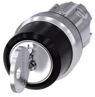
RONIS key-operated switch, 22 mm, round, metal, shiny, lock number SB30, with 2 keys, 3 switch positions I-O<II, left latching, right momentary contact type, actuating angle  $2x45^{\circ}$ , 10:30h/12h/13:30h, key removal O+I, possible special locks: SB31, 421, 455
