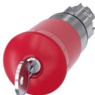
EMERGENCY STOP mushroom pushbutton, 22 mm, round, metal, shiny, red, 40 mm, with lock Siemens, lock no. SSP9, positive latching, according to DIN EN ISO 13850, key-operated release
