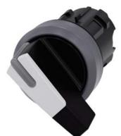
Selector switch, illuminable, 22 mm, round, plastic with metal front ring, white, selector switch, long, 2 switch positions O-I, latching, actuating angle 90°, 10:30h/13:30h
