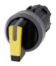
Selector switch, illuminable, 22 mm, round, plastic with metal front ring, yellow, selector switch, short, 3 switch positions I>O<II, momentary contact type, actuating angle  $2x45^{\circ}$ , 10:30h/12h/13:30h
