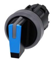
Selector switch, illuminable, 22 mm, round, plastic with metal front ring, blue, selector switch, short, 3 switch positions I-O-II, latching, actuating angle 2x45°, 10:30h/12h/13:30h
