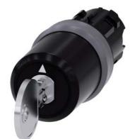
Key-operated switch BKS, 22 mm, round, plastic with metal front ring, lock number S1, with 2 keys, 3 switch positions I-O<II, left latching, right momentary contact type, actuating angle  $2x45^{\circ}$ , 10:30h/12h/13:30h, Key removal O+I
